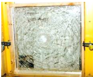
Broken laminated glass.
